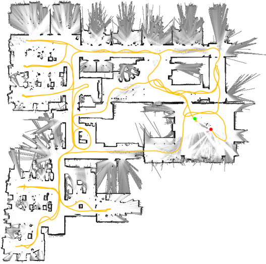
Fig. 5. Cartographer map generated using Revo LDS sensor data.
